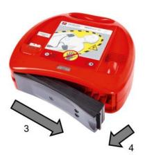
Fig. 10: Removing the battery
